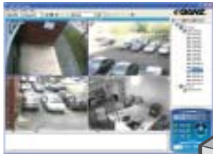
PC running client software allowing live, playback, PTZ control, programming & event archive of the DVR via LAN or WAN.
