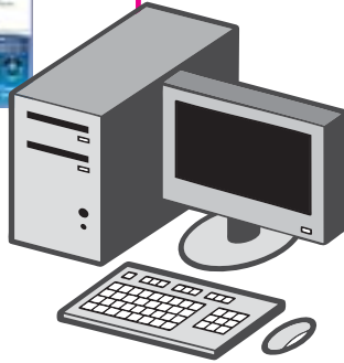
PC running client software allowing live, playback, PTZ control, programming & event archive of the DVR via LAN or WAN.
