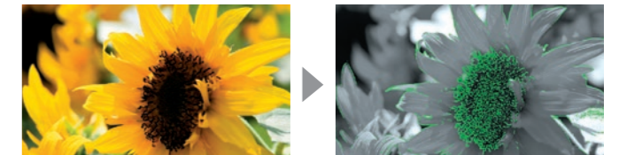
When the Focus Assist function is set to ON, objects that are in focus appear with colored edges (selectable from red, green or blue) as seen here.
