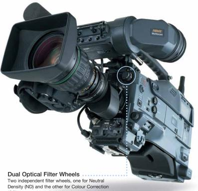
(CC), are provided. An optional servo filter drive unit, the BKDW-701, can also be fitted allowing filter settings to be changed with the RM-B750/150 Remote Control Unit.
